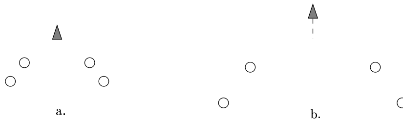
Figure 7.4: The triangle represents the leader, and the circles the positions of \mathbb{P} . If the vehicles did not have a common unit distance, then they could scale \mathbb{P} , and the flock would not follow L while it moves.
